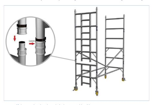
1.6 Make sure that the trigger is facing to outside of frame.
