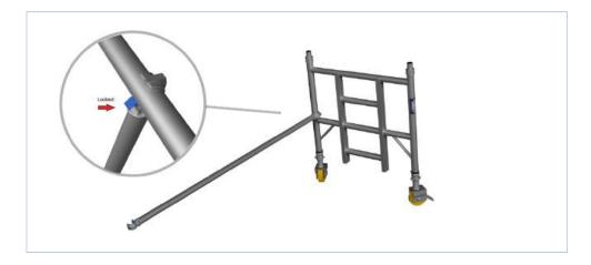
1.4 Position the ladder frame as shown and fit the other end of the horizontal brace onto the vertical.
