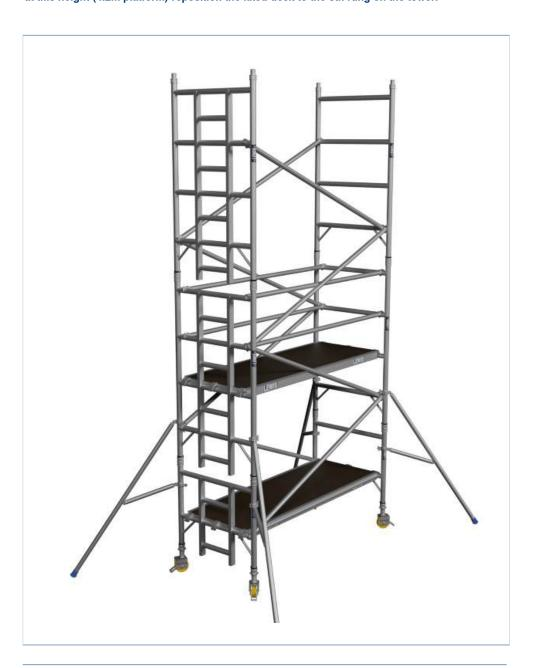
1.11 Add two more diagonal braces between the 5th and 7th - 7th and 9th rungs. If finishing at this height (4.2m platform) reposition the fixed deck to the 8th rung on the tower.
