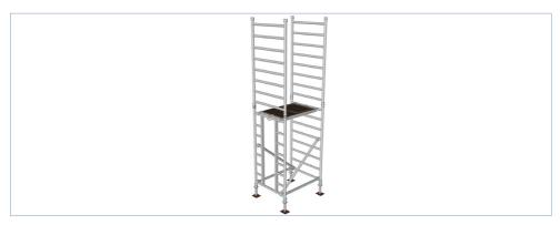
6. Fit diagonal braces (blue trigger) from bottom frames to bottom rungs of top frames.
