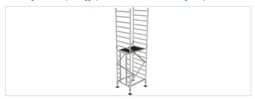
7. Fit 4 horizontal handrails above platform (500mm and 1000mm). Fit 2 more diagonal braces as pic.
