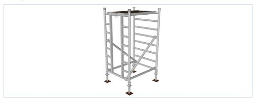
5. Fit frames and secure frames with locking frame clips.
