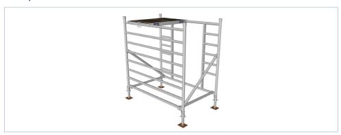
5. Fit frames and secure frames with locking frame clips.
