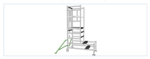
8. Pull the gate into the closed position – You must ensure the gate hook is securely fastened, and locked into place. Do not use a podium if you are unable to secure this gate.
