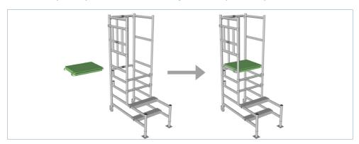
5A. If the podium platform is variable, please ensure the correct handrail bar is put in place to ensure that the total height of the handrail is 950mm
