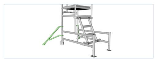
7. Pull the gate into the closed position – You must ensure the gate hook is securely fastened, and locked into place. Do not use a podium if you are unable to secure this gate.
