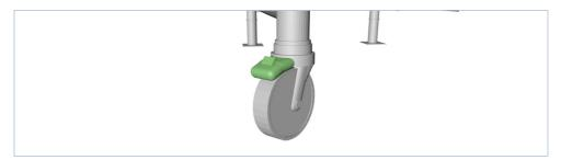
7. If your Podium has Stabilisers – Fit the stabilisers at a 45 degree angle. If you are unable to do this, due to the placement of the podium place the stabilisers parallel.
