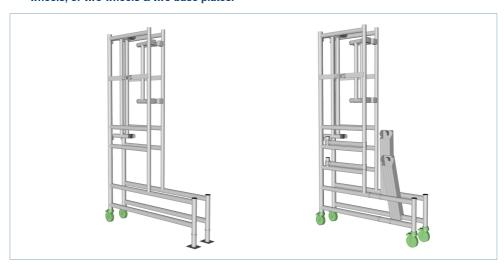
2. Open the podium frame and unlock the elbow - ensure they are locked into position securely
