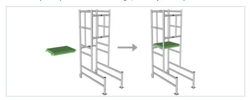
3A. If the podium platform is variable, please ensure the correct handrail bar is put in place to ensure that the total height of the handrail is 950mm
