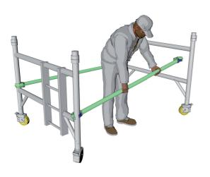
NOTE: Check all brace claws are positively locked after fitting.
