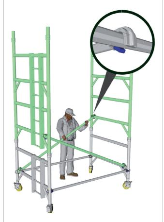
IMPORTANT- Only use the adjustable legs to level the tower and not to gain extra height. Adjustable legs should only ever be extended to minimum amount required to level the tower.
