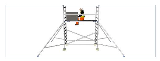
1.21 Climb internally up the rungs of the frame through the trap door platform. site with feet through the platform, so they are resting on the rung of the frame. Fit four guardrail braces on the 2nd Rung and 4th Rung above the platform. or at approx. 250mm above the platform, then a further 250mm from there.
