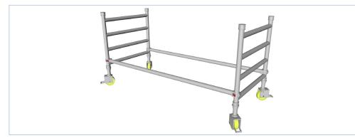
**1.7** Make sure the Trigger is facing the outside of the frame.
