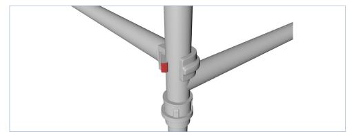
1.8 Insert the next section – this may vary in size depending on which tower you have. However, the image we have used, is an 8 Rung (2m high) frame.
