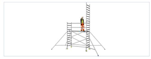
1.26 Stand on platform and ensure the guardrails are securely in place at the opposite end of the tower.
