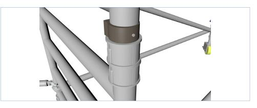
1.18 Attach the trap door platform approx. 2.2m above ground level. This will be on the 8th Rung, if you started to build the tower with an 8 Rung Section. If you started to build the tower with the 4 Rung (1m) frames, then the 1st platform will be placed approx. 4 Rungs above the frames. This will vary depending on what section you have started to build your tower with.
