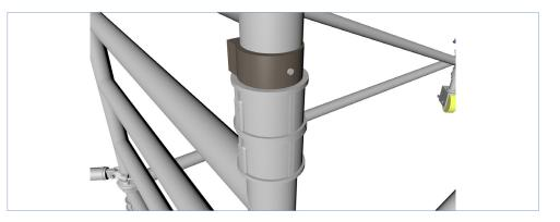
1.28 Place the trap door platform approx. 2m above where you are standing. The platform should now be placed approx. 4.2m off the ground. Our images show, the second platform is placed at a 4.2m platform.
