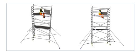
1.33 Stand on the platform to inspect and check the braces are all securely into place, and facing the correct way.
