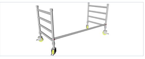
1.6 Clip the second brace in the same position, on the other side of the frames. Make sure the base is level using a sprit level. Any alterations needed, can be adjusted on the legs.
