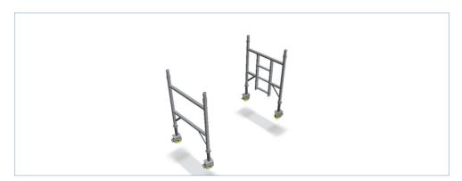
1.5 Clip horizontal brace onto span frame. Connect the brace directly above the casting at the first horizontal rung position. And then attach to ladder frame.
